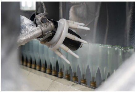
In the new liquid coating system, the first step is to process the glass bottles with the GA 1030 automatic airspray guns.
