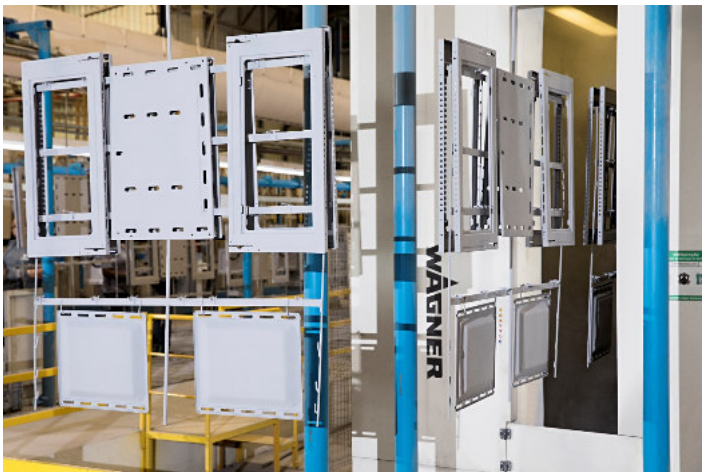
Enameled workpieces coming out of the powder booth
