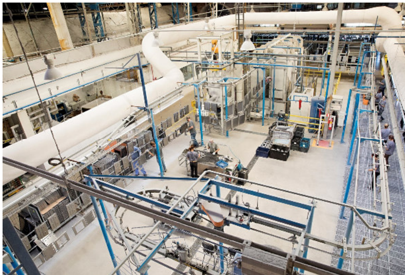
Overview of the workshop with workpieces entering the powder booth.
