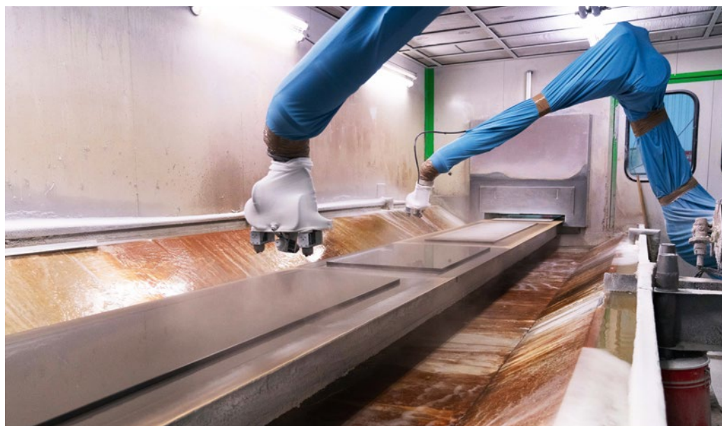
The use of high-pressure double-diaphragm pumps has also improved the spray pattern of automatic paint application at Neelsen GmbH.
